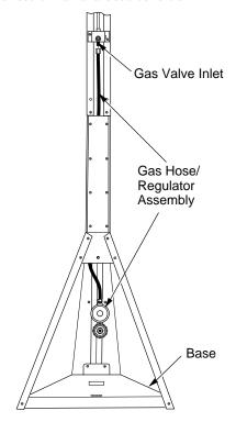
Figure 9 - Installing Hose and Regulator Assembly
